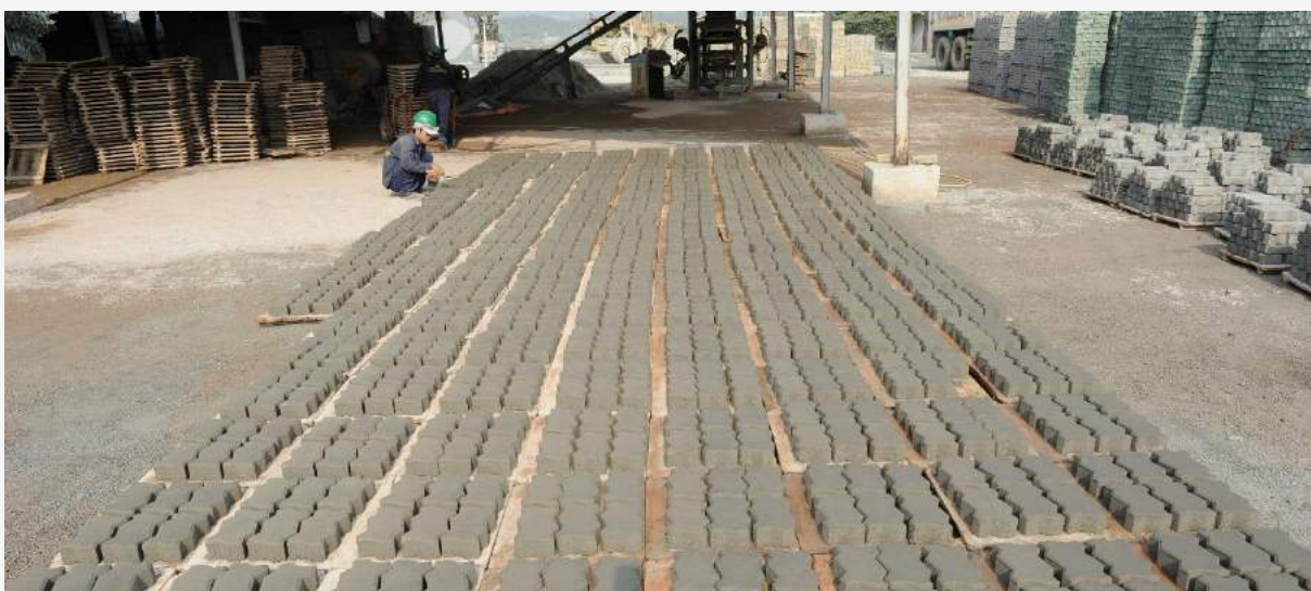
PRODUCTION OF INTERLOCKING CONCRETE BRICK
