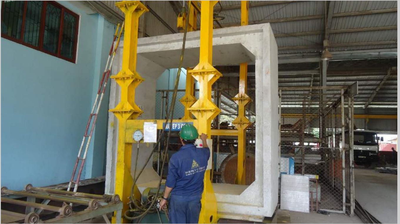
The culvert products are tested by triaxial compressor certified by Quatest 3
