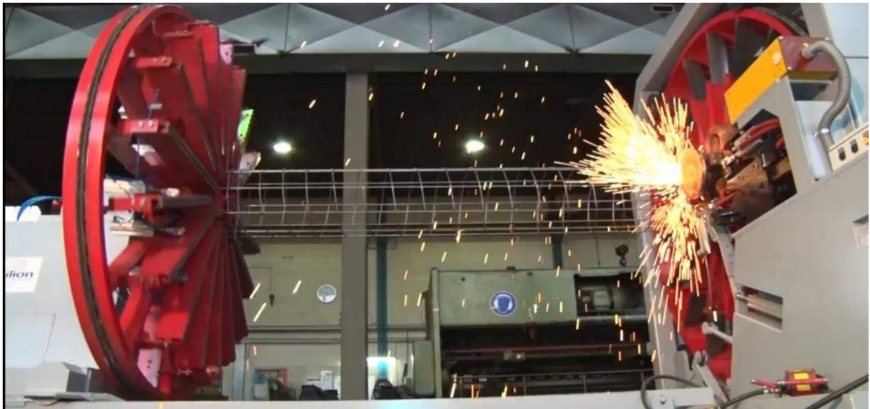
Automatic steel pipe culvert welder and culvert forming mold
